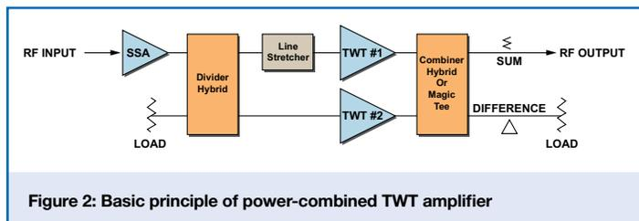
Besides providing higher output power, power combining TWTs improves reliability by providing graceful degradation. In other words, the failure of one amplifying device will not bring down the entire transmitter. Reliability improvements also result from lower operating voltages, modularization, better thermal management, and reduced stress levels on components.
