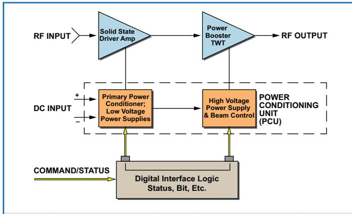
**Figure 3: Microwave Power Module (MPM) block diagram**
